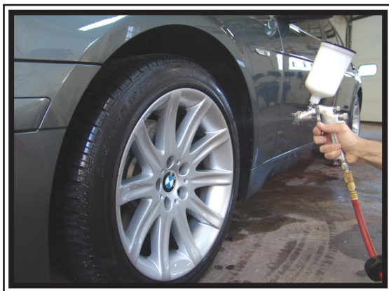
Above: With a spray gun, you can "paint" dressing on the tires without getting it on the wheel or the painted surfaces.
