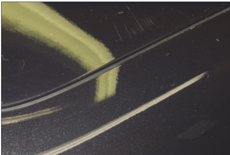
In the above picture the "orange peel" appearance in the paint can clearly be seen.
