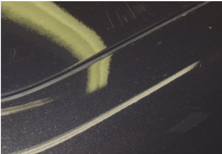
In these pictures, the “orange peel” appearance in the paint can clearly be seen. The reflection of the overhead fluorescent light accentuates the problem in both photographs. This vehicle happens to be a new Mercedes E class. You wouldn’t think a Mercedes would have a look like this, but this is what most factory paint jobs look like up close.
