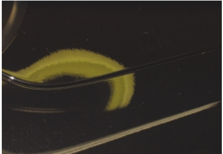
In these pictures, the “orange peel” appearance in the paint can clearly be seen. The reflection of the overhead fluorescent light accentuates the problem in both photographs. This vehicle happens to be a new Mercedes E class. You wouldn’t think a Mercedes would have a look like this, but this is what most factory paint jobs look like up close.
